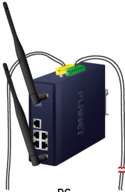
DC Power Failure
